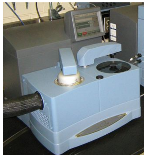
Figure 31. DSC Q2000 TA Instrument as used for thermal analysis of iodine-doped radicals and metal-radical complex. Picture from Professor Dmitriy Soldatov's website.
