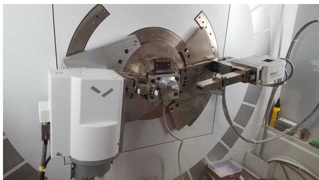
Figure 24. PXRD machine (nickname “Panda”) used for sample measurement, set up with a spinning capillary tube in the centre for the sample. The right “arm” of the machine is capable of rotating to measure the diffracted x-rays for the angle range specified.
