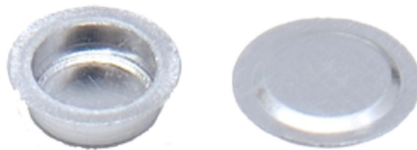
Figure 30. T-zero aluminium hermetically-sealed pan (left) and lid (right) for DSC measurement of air-sensitive materials.
